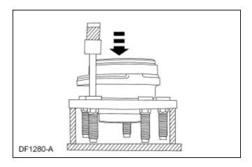
2. Install the wheel bearing and hub assembly. For additional information, refer to Wheel Bearing and Wheel Hub in this section.
